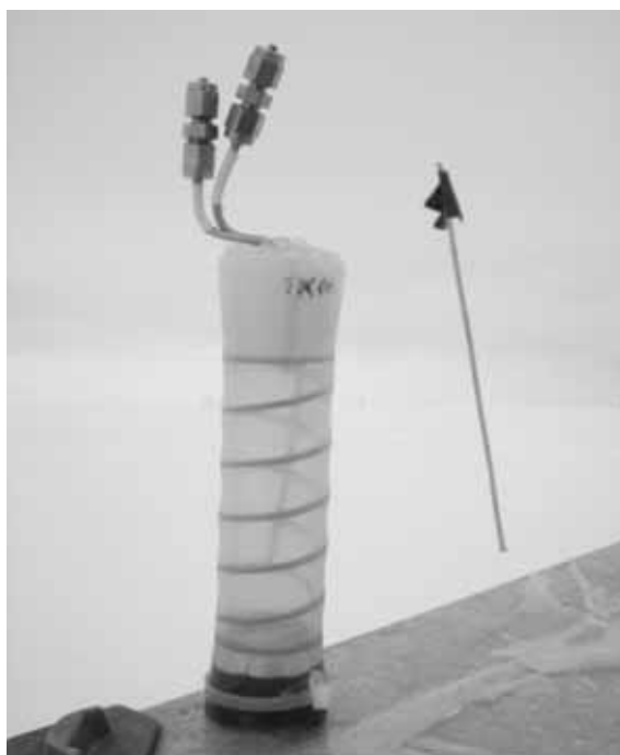
Figure 2 Silicone chamber known as peeper for sea ice p\text{CO}_2 measurements.
