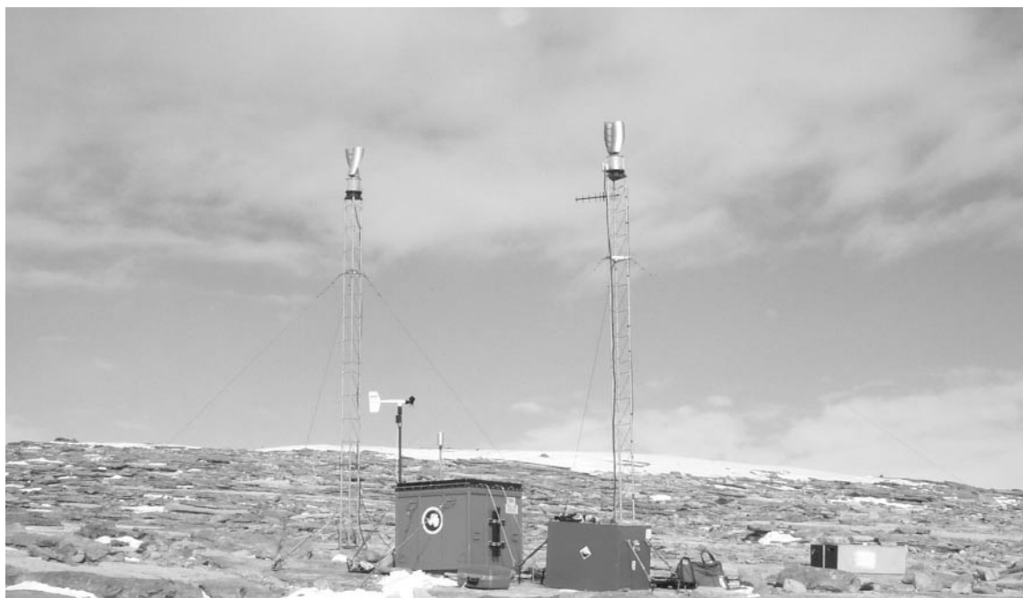
GPS installation at Mt. Coates, located in the Dry Valleys. Photograph Courtesy C. Raymond, JPL/NASA.
